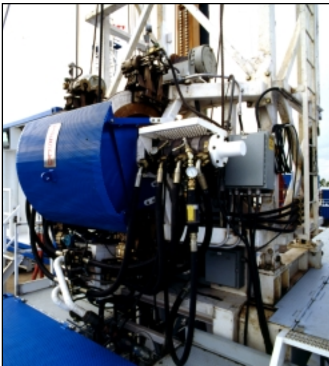
Fig. 5. Drawworks and mast integration.
